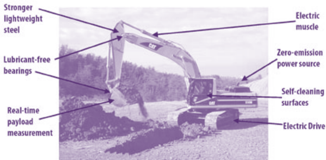
Figure 3.2. Productivity enhancements envisioned for CAT heavy equipment through nanotechnology (courtesy of Caterpillar Inc.).
